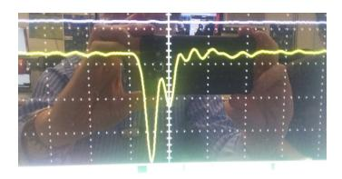
**Silicon signal**: 24ke/mip/300um, amp.gain x400, pulse width 5ns (base) From capacitance (17pf) and area (36mm2) it looks like the effective diode thickness is 220um (Si dielectric constant is 11.7), so the charge should be about 18Ke/mip ?????????
