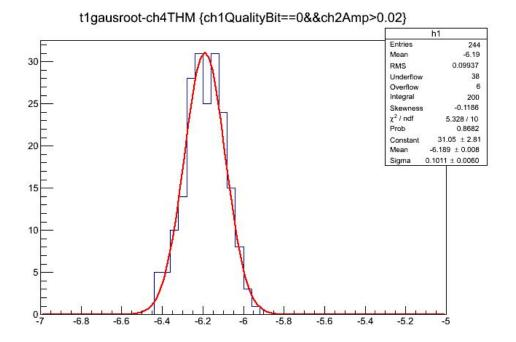
Run 055: electron 8 GeV taking data with 1.7cm LYSO with 3mm2 SiPM. SiPM HV at 71 V. Seems like the signal on reference Ham is too small, may affect the resolution. Decide to increase the HV to 3.0 kV. Stop the current run and move Ham A up.
