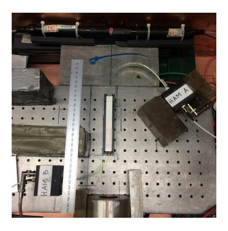
Run 083: Shashlik cell with dual readout, 12 GeV electrons. Ham A and B HV = 2.8 kV.
