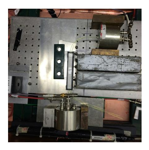
Run 051: setup as shown above, DSB1 fibers. Electrons @12 GeV. We get decent energy peak ( $\sim$ 8%) and  $\sim$ 350 psec time resolution, shown below. The run declared a very good run.
