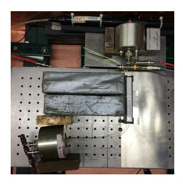
Run 049: electron 12 GeV with the setup above. Goal is to see if the spike on rising edge is removed.
