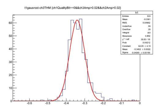
Run 065: 32 GeV electrons, Ham B 20 dB attenuator. Ham A HV = 3.0kV, Ham B HV = 2.8 kV. 1.7 cm2 LYSO Ham B. Pressure is put at 1.25psia. We get around 35 psec.
