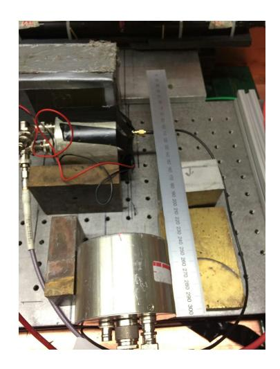
Run 042: electron 12 GeV beam, triggering on SC counters, as normal. Collect some data with this, and then change the SiPM capacitance to 10pF again, seems that produced the best rising edge. We get TOF resolution between PHO A and B around 50 psec. We hypothesize that in May TB we had the reference upstream of LYSO, and could have had showers hitting the LYSO producing more light. We will test this hypothesis next CA.
