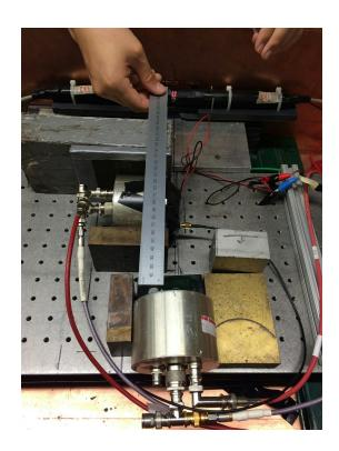
Run 041: trigger on CH3 AND CH4, SiPM at 67.5V. This is more of a commissioning run to see how the pulses from the SiPM and amplifier look.
