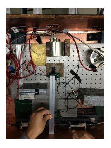
Run 044: electron 12 GeV. We seem to be still not aligned with the trigger. Continue taking events triggering on CH3. SiPM HV = 70 V.
