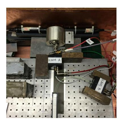
Run 073: Shashlik cell with single readout. Ham A and B HV = 2.8 kV. Pressure is 1.0 psia. Photek A HV = 4.9 kV. We observe that there is no dual peak between Photek and Hamamatsu A, so Photek can be used a reference detector. TOF resolution between Ham A and Ham B is  $\sim 300 \text{ psec}$ , similar results for Photek, consistent with previous run.
