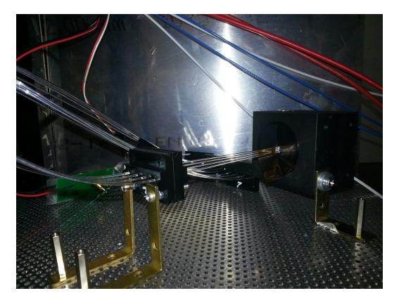
Fiber connector (top right, with two fibers going in from the back. Bottom left : Diffuser for SiPM coupling in the default SH matrix setup - not used by us for now.) :
