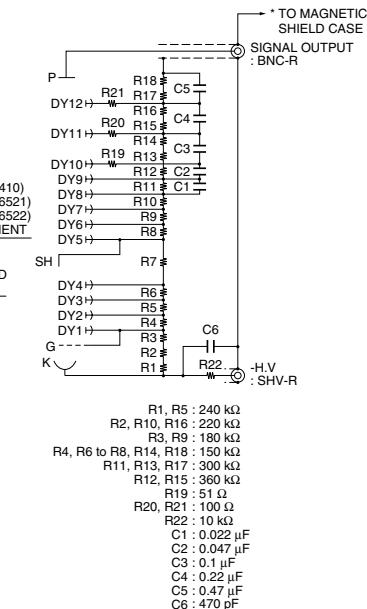
\* MAGNETIC SHIELD IS CONNECTED TO GND INSIDE OF THIS PRODUCT.
