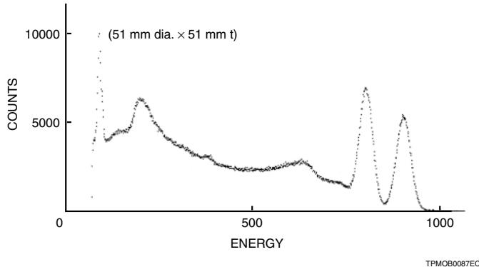
By analyzing these output pulses using a multichannel analyzer (MCA), pulse height distribution (PHD), or energy spectra, as shown in Figure 32, are obtained. From the PHD, the number of incident particles at various energy levels can be measured.
