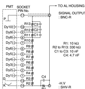
The housing is internally connected to the GND.
