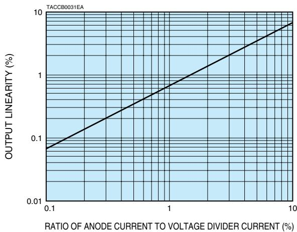
As stated above, good output linearity can be obtained simply by increasing the voltage divider current. However, this is accompanied by heat emanating from the voltage divider. If this heat is conducted to the photomultiplier tube, it may cause problems such as an increase in the dark current, and variation in the output.
