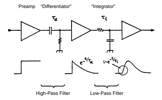
Simple arrangement: Noise performance only 36% worse than optimum filter with same time constants.
