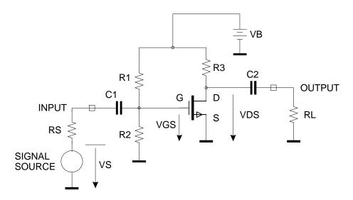
First, just consider the DC operating point of the circuitry between C1 and C2:
