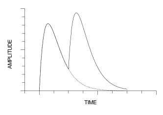
Reducing pulse shaping time to 1/3 eliminates pile-up.
