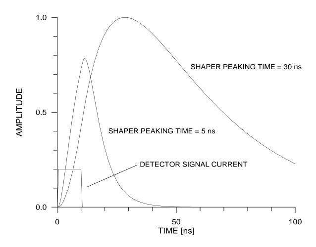
Note that although the faster shaper has a peaking time of 5 ns, the response to the detector signal peaks after full charge collection.
