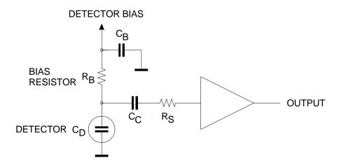
Detector bias voltage is applied through the resistor  $R_B$ . The bypass capacitor  $C_B$  serves to shunt any external interference coming through the bias supply line to ground. For AC signals this capacitor connects the "far end" of the bias resistor to ground, so that  $R_B$  appears to be in parallel with the detector.
